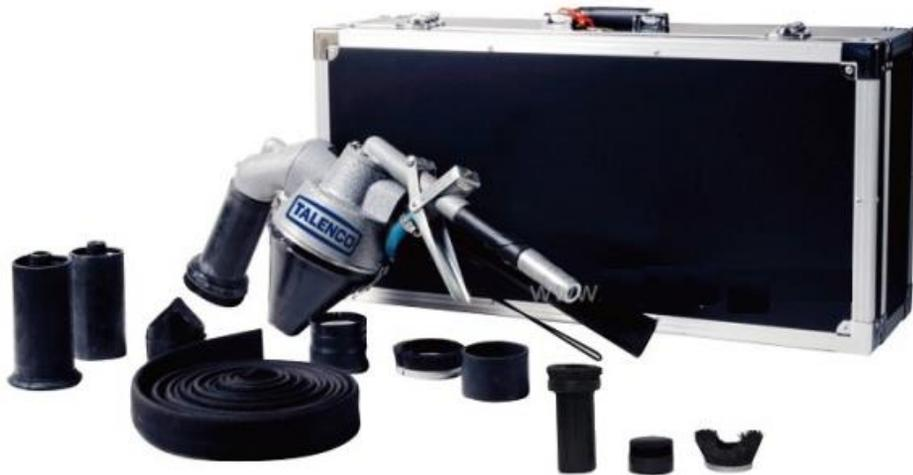
**Portable Dust Free Blast Machine** is a light-weight , portable abrasive blasting tools with an integral abrasive recovery system. During Blasting , abrasive is continually recycled , while dust and other debris are collected in a slip-on dust bag Interchange adapter boots for level surfaces , corners, etc. fit over the swivel blast head to assure efficient recovery on any surface
